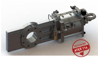
CONEX IVM is used to monitor the basic status of GatEx and manual closing or opening. Information about the increased explosion pressure subsequently continues to the control unit CONEX, where the signal is evaluated as an explosion. Conex then sends a signal again via CONEX-IVM to the GatEx quick-release valve, which by moving it from the initial position causes the compressed air to blow out of the air into the pneumatic cylinder, thereby closing the GatEx
